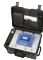
SF 6 gas analyzer
